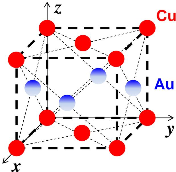
2 Cu atoms and 2 Au atoms per unit cell
