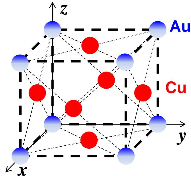
3Cu atoms and 1 Au atoms per unit cell
